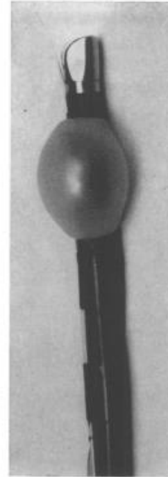
FIG. 2. Head of instrument with balloon inflated for bringing mucosa into focus, and cannula protruding in front of lateral lens.
